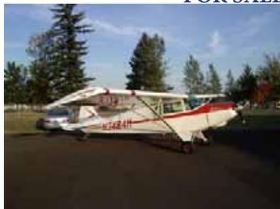
4132 Hrs TTAF, 160 HP, O-320A2B, 560 Hrs SMOH, B&C Starter, B&C Alternator, Borer Prop, Super Cub Tail, Flaps, Booster Tips, long-range tanks (61 gallons total fuel), Float Fittings, Lifetime sealed struts, KLX 135 GPS/COM, KT 76A Transponder, Night VFR panel, PS 1000 II Intercom, Attitude Indicator, EGT/CHT Gauge, Strobe Lights, Landing Lights, Extended Baggage, 8.50X10 Wheels and second set of 6.00 X 6 wheels.
