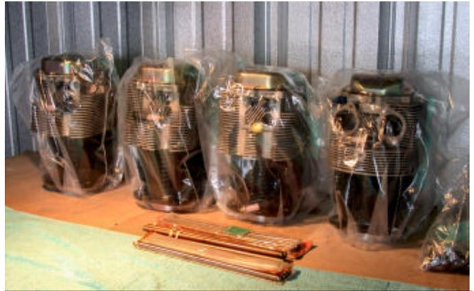
*New Superior cylinders staged for installation in RV-8 N558RL.*
