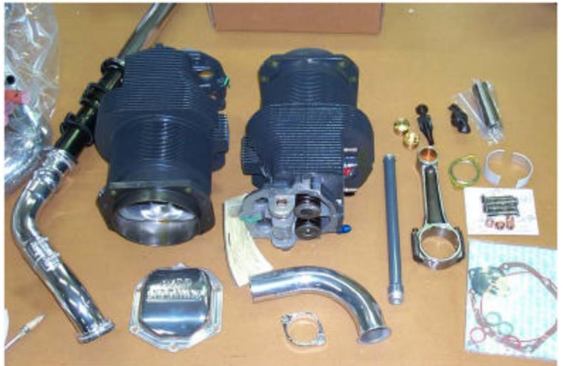
one cylinder, from the connecting rods to the exhaust. Notice that I had some parts Ceramic coated. Whether or not this is a good idea will have to be proven over time, but the basic reasoning is that it will keep the heat in the pipes and exhaust it out the ends, with less radiation of the heat into the engine components and cowl.
