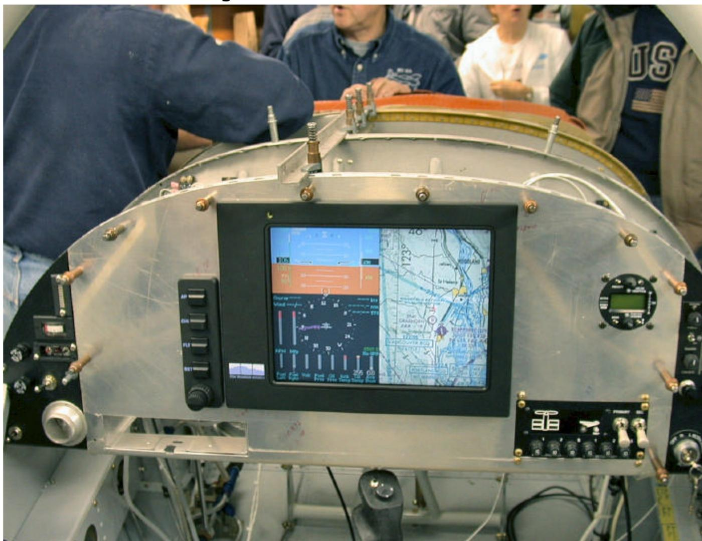
*Harmon Lange goes state-of-the-art with his new RV-8A, panel pictured above. Not only has he installed the Blue Mountain Avionics EFIS system, but has an Aerosance FADEC system on his new Aero Sport Power O-360.*
