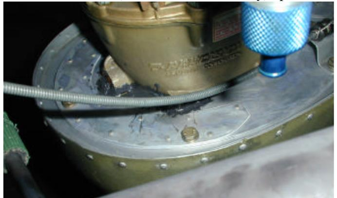
tween the plate and carb, so the plate will clear the ridge/step without having to notch. I've also seen people machine this casting and shoulder flat. Taking off the casting ridge seems okay to me, but I personally would be a little hesitant to machine down the shoulder on the carburetor.
