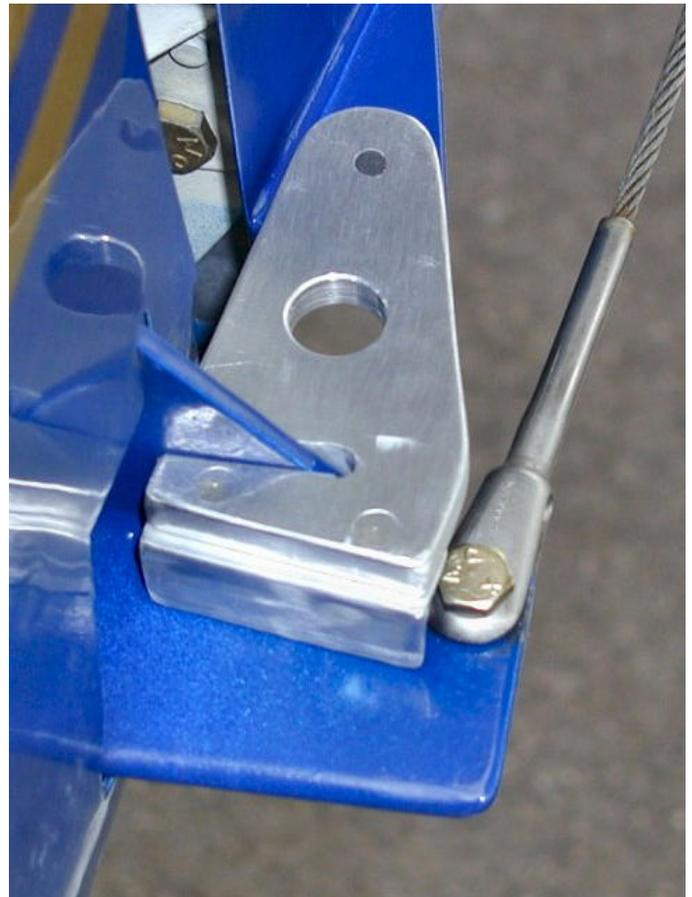
thread-locker. A hacksaw removes the bolt head and the excess threads. When cutting the slot, note that it is not quite perpendicular to either axis of the bar stock. The key is to make sure the body of the lock lays flat against the top surface of the rudder stop so the pin will remain secure in the hole drilled there. With a little planning, and plenty of filing, it isn't too difficult to get everything to fit.
