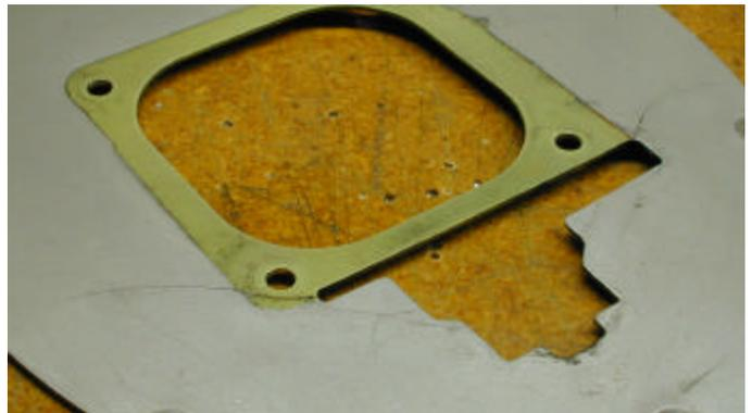
Made a new plate, and added a U-shaped reinforcing piece in the affected area. A better way to deal with this would be an .063 (or as thick as necessary) spacer be-
