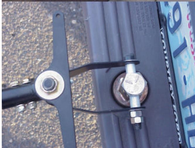
**TOP:** Randy Griffin's fuselage prepares to go 35 mph in reverse. Note the bicycle strobe attached to the engine mount. **BOTTOM:** Randy's copy of Larry's design. To allow the fuselage to move longitudinally relative to the tow vehicle, Randy slotted the post where the cross bolt goes through... worked great.
