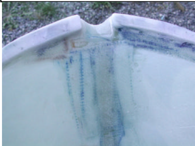
BELOW: the fiberglass work on the inside rear of the skirt.
