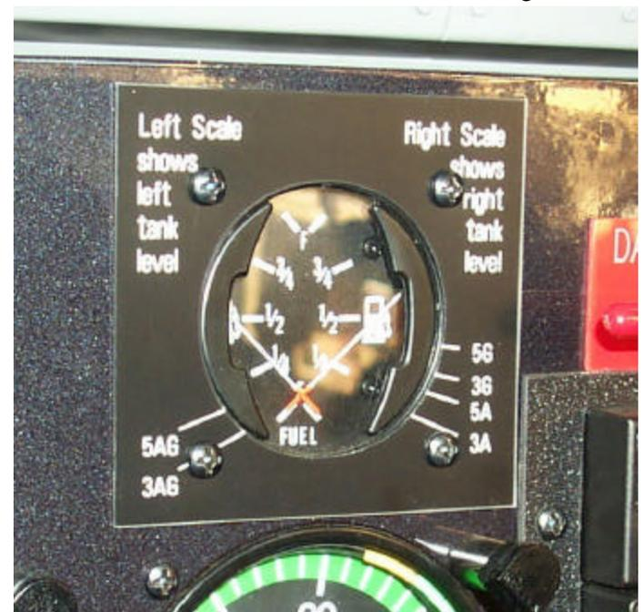
the needles didn't match side to side nor to the scale on the gauge. Notice that A = Air and G = Ground. The left tank is the aerobatic tank with the sender located thru the rear baffle in the second bay, and it doesn't change between tail low or flying attitude for the taildragger RV-6. The standard right tank has a big difference. Let me know if you're interested in getting one of these, I have the cad dwg and can get them made at my local engraver.
