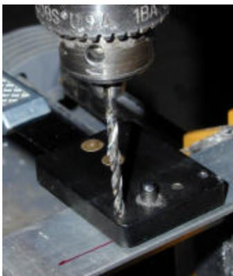
6. deburr screw hole and countersink rivet holes—usually takes me 4 revolutions
