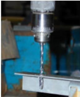
1. drill full-sized hole for #8 screw, #19 drill bit
