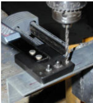
4. flip jig over, use set of posts to position jig for drilling second rivet hole
