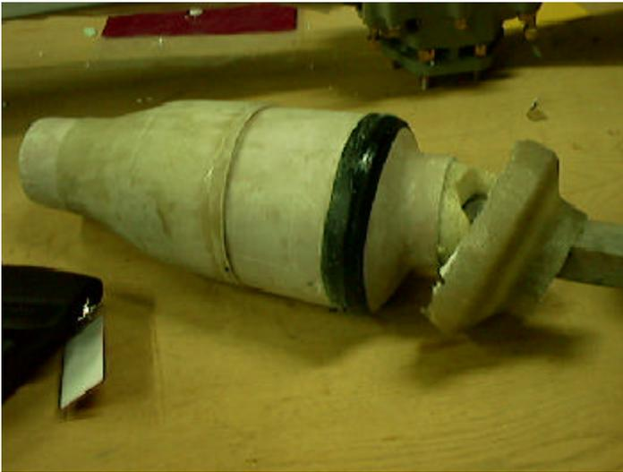
Almost finished pieces and mold for The Duck's Air Filter Housing.
