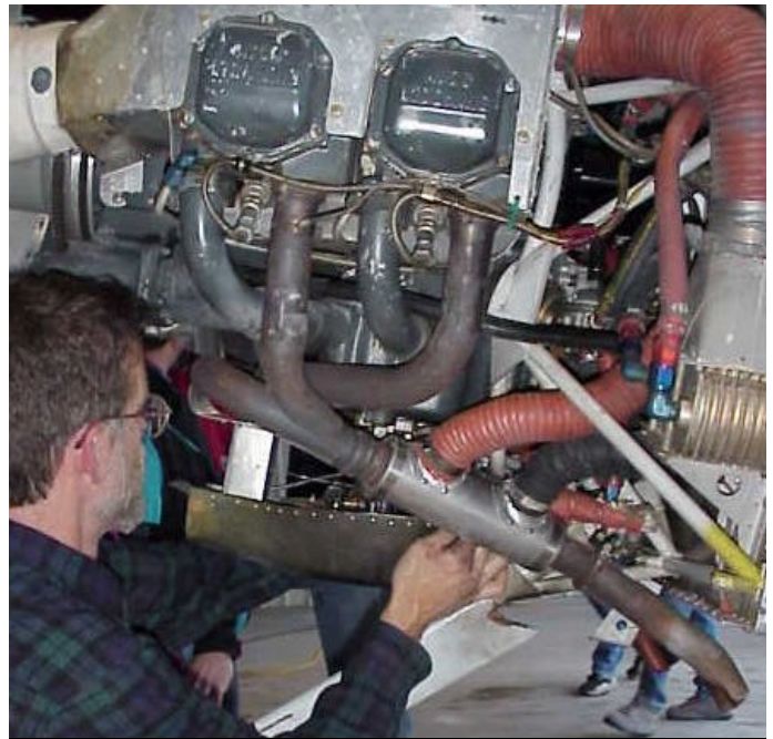
Kevin checks for damage to his airbox after his induction system fire – fortunately there was very little!
