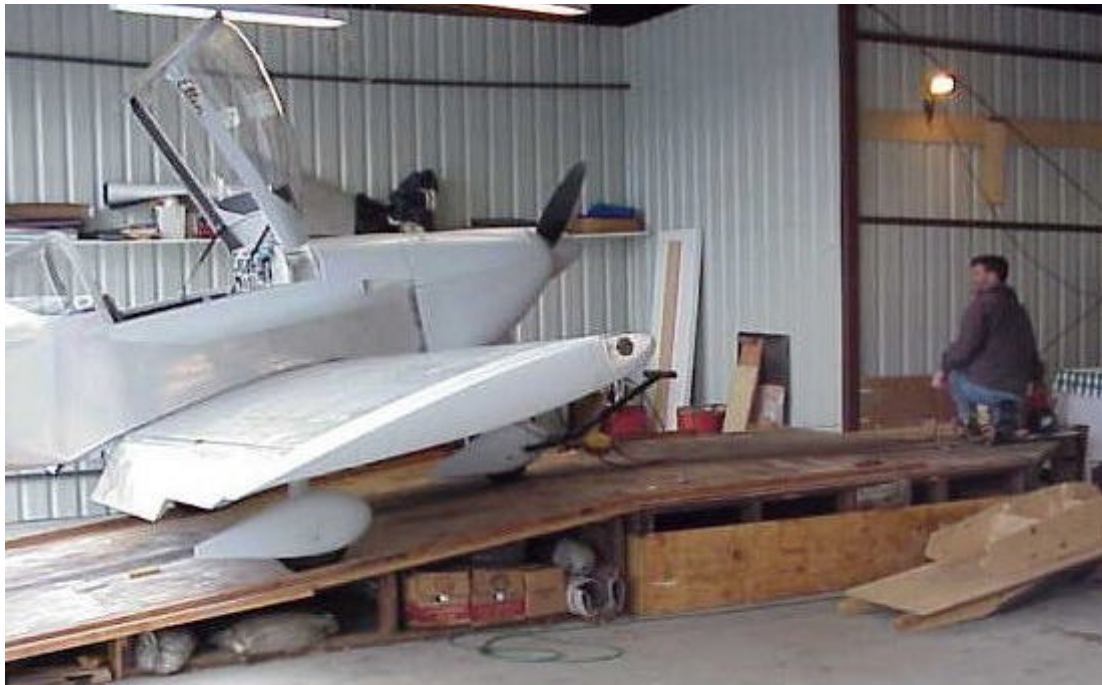
This is how Kevin and Brian manage to keep TWO RV-6As in one normal t-hangar. Here is Kevin using his motorized winch to bring N3773 up onto the storage ramp after his induction fire.
