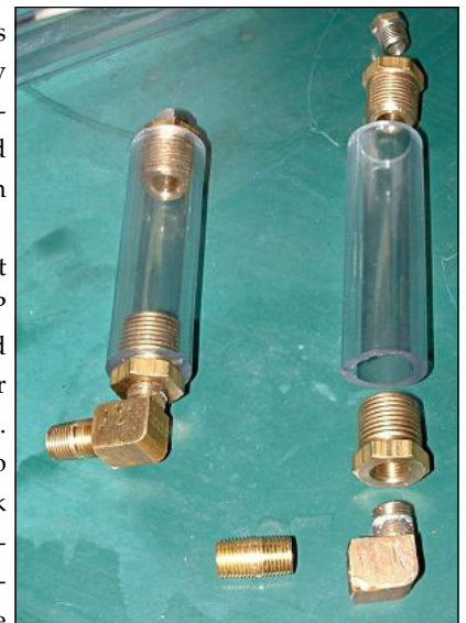
Test-assemble the clear brake fluid reservoirs without the pro-seal.
