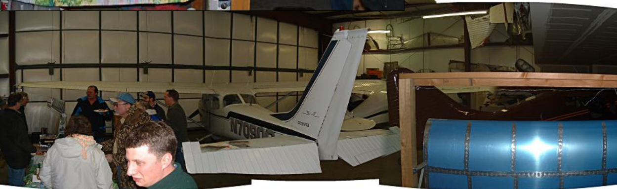
Right: The wing jig Kent uses is on wheels to accommodate all the airplane traffic in the hangar.
