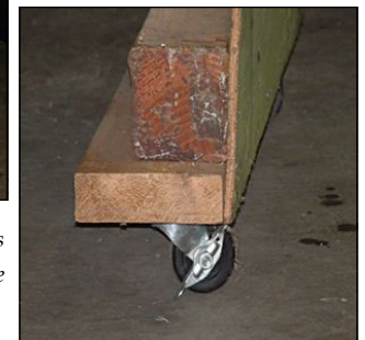
Right: The wing jig Kent uses is on wheels to accommodate all the airplane traffic in the hangar.
