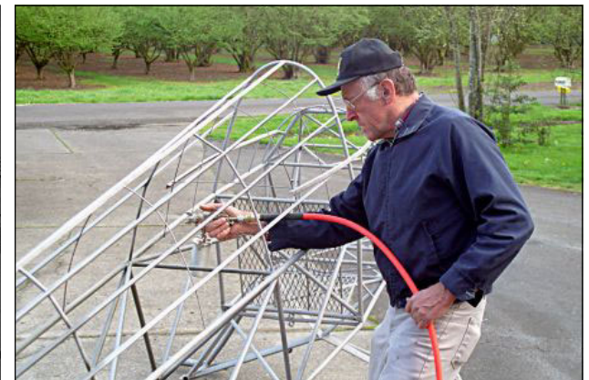
Stan VanGrunsven applies wash primer to the Bogardus Little Gee Bee fuselage.
