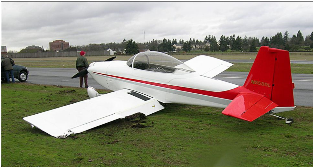
RV-8 N558RL at rest after encountering a gusting cross wind at the wrong time.
