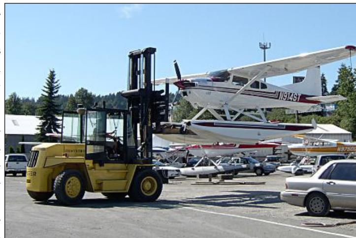
This is how the seaplanes are taken from the water ramp to their tie down positions. In this case the seaplane has already been lowered to about the 60% level. It had been raised about half again higher to clear the flight office when it was first removed from the water ramp. Photo: Don Hammer.
