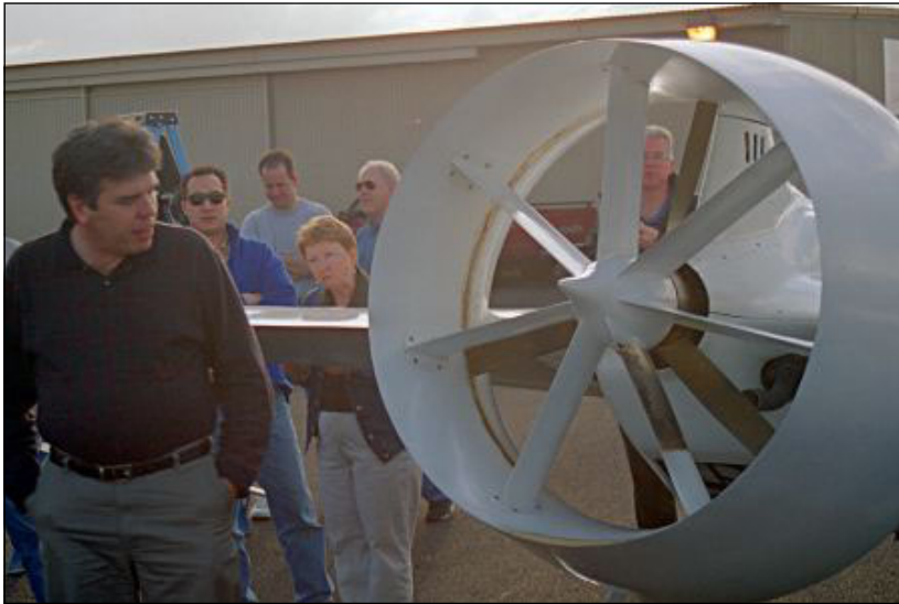
Left: Perry Mick presents his Ducted Fan Long EZ. The fan is only half of the unusual power system. The Mazda 13B Rotary engine is directly driving the fan with no gear reduction. Right: Al Wick talks about his Subaru powered Cozy Mk-IV. Al has the aircraft extensively instrumented and also carves his own props.
