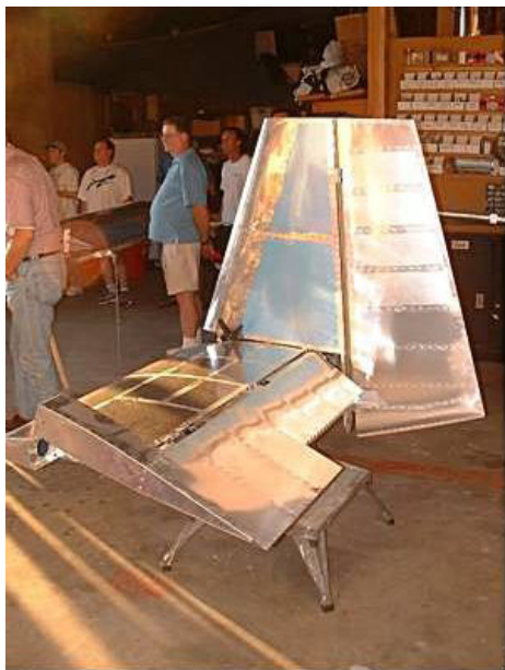
Thin Skinned, the airplane is built almost entirely of .016.
