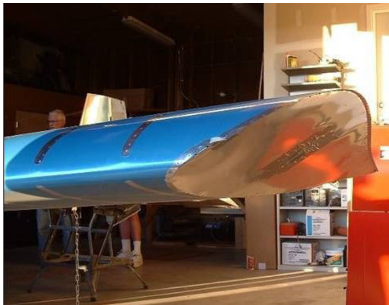
NO FIBER-GLASS! At least as little as possible. Check out these all-aluminum wing tips!
