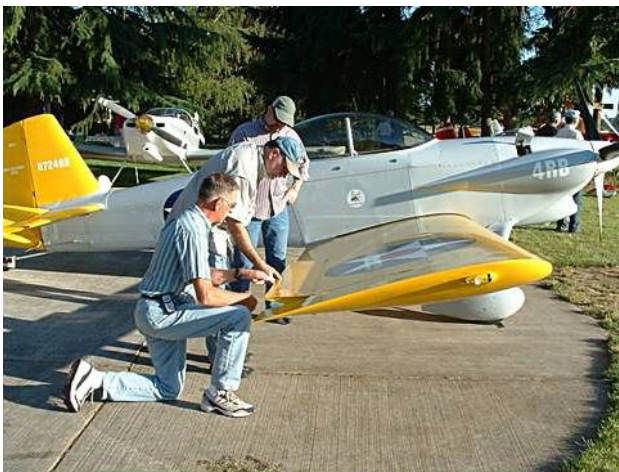
RV-4 inspection — Jerry VanGrunsven, Rion Bourgeois and Bob Neuner critique aileron adjustments.
