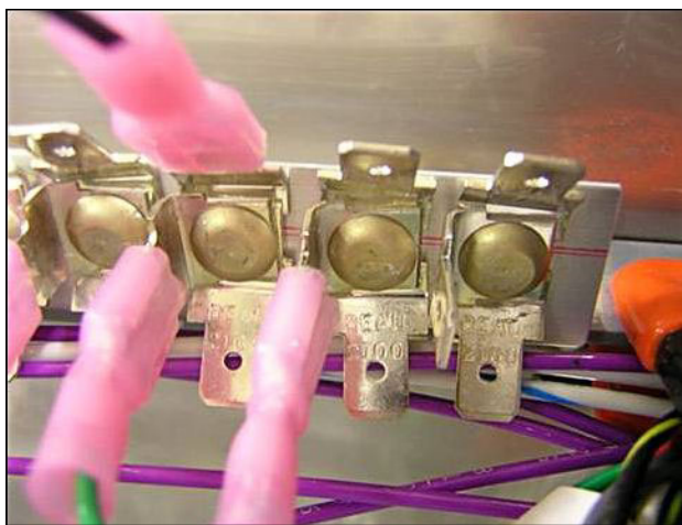
This custom ground block cost less than $5 for 36 tabs.
