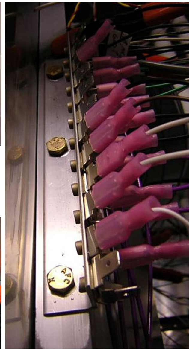
This custom ground block cost less than $5 for 36 tabs.
