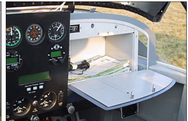
A tidy map-box installation. If this were a Mustang, would it be a jockey box? Photos: Kent Byerley.
