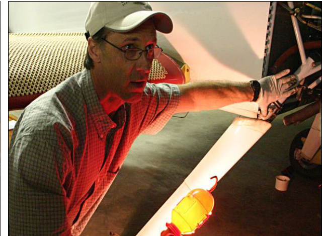
Gear leg and engine mount inspection.
