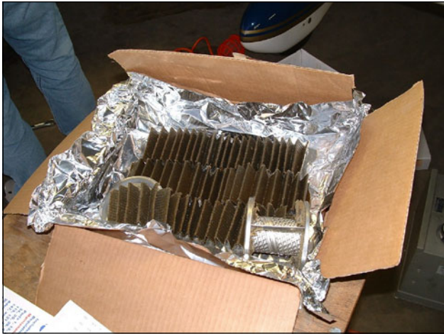
Oil filter cut open for inspection. A magnifying glass and a magnet are useful tools at this stage.
