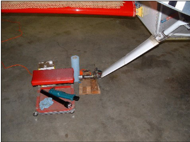
Up on blocks, the wheel spindle is cleaned, inspected and given a light coat of grease. The brake pads are inspected and cleaned or replaced and the brake caliper is cleaned and inspected.
