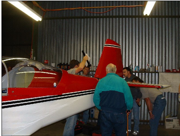
Empennage attach inspection. Missing something here can really ruin your day.
