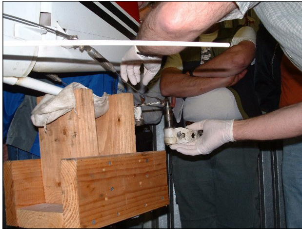
Tail wheel fork pivot inspection and lubrication.
