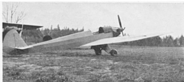
Side elevation of the Low-Wing Longster showing the fuselage fairing methods and the landing-gear streamlining.
