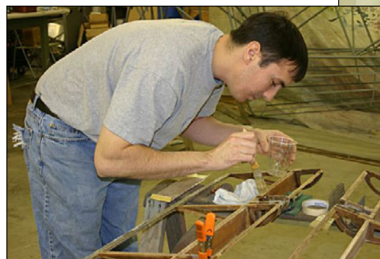
A few pictures from the Little GEE BEE work party at DickV's Sunset Shop, Saturday, Jan 29th. Around ten people turned out to work on repairing wing ribs, and sanding woodwork in preparation for varnishing.
