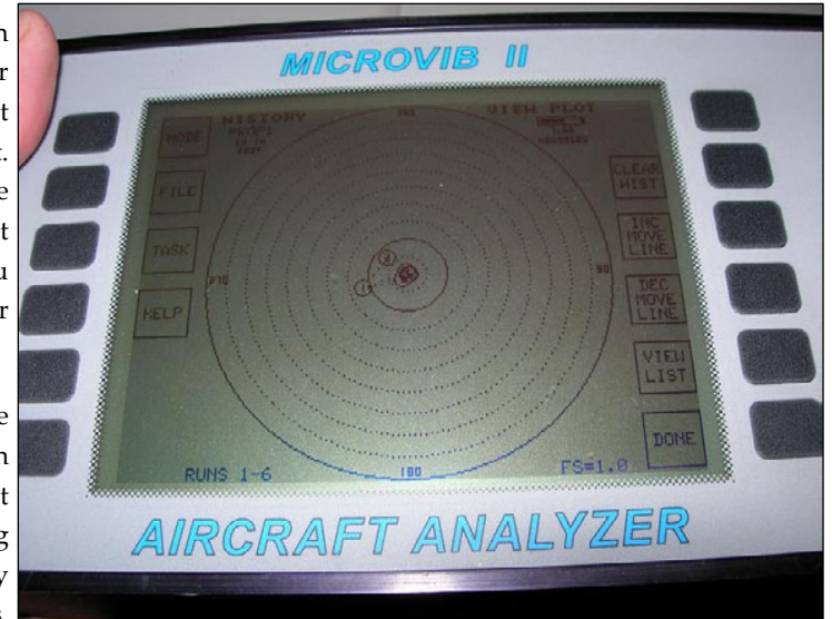
Polar plots of successive balance runs. Once you're inside the smallest circle you're just shooting for bragging rights.
