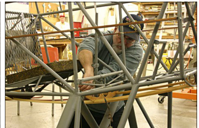
The aileron: open (fabric) bays with aluminum leading edge; Dick V checks the fit; Tom Story wrestles with control stick cable fittings.
