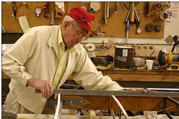
Photos continued from pg. 6. Ken checks spanwise straightness, sands to even.
