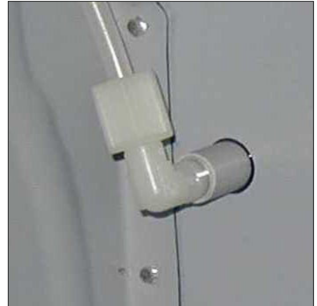
AN RV STATIC VENT INSTALLATION THAT PROVIDES FOR ATTACHMENT OF A STANDARD 1/8 NPT TUBE FITTING
