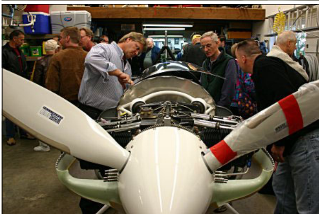
The engine was built by Aeroport Power in Kamloops, BC, Canada and uses Precision Airmotive fuel injection. It spins a light (28 lb) Whirlwind model 151 constant-speed prop.
