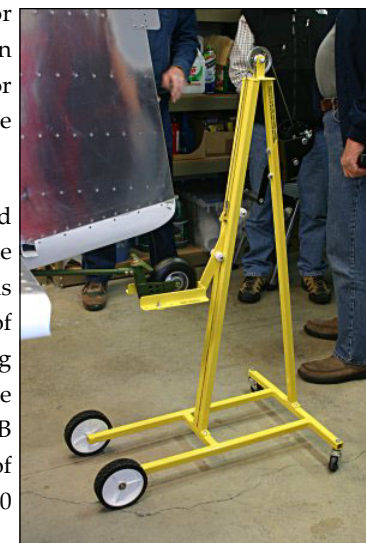
Randy likes his tail lift. Many operations require the plane to be leveled, and the winch saves his back.
