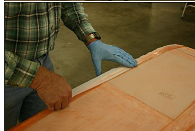
Dick VanGrunsvon and Louise Lane worked the June 4 session, applying tapes and inspection rings to the Bogardus Little GEE BEE restoration project.
