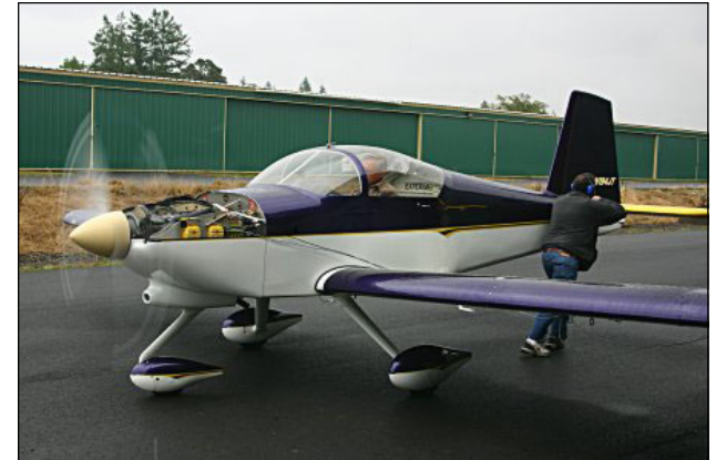
Above: Jake Thiessen receives a prop balance-treatment on his RV-9A. Opposite corner: Randy Griffin, Bill Drake and Randy Lervold — the Randy's team up to balance Bill's RV-6 prop, explaining the process as they go.
