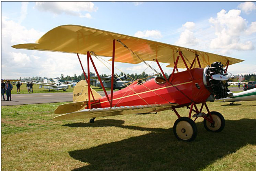
Phil Taylor's 1930 TravelAir 4000 (NC426W). Mounts a Lycoming R-680 of 300 HP. The airplane cruises in the 100-105 MPH range, and lands at around 45-50. Photographed at the 2005 NW-EAA Fly-In, Arlington.
