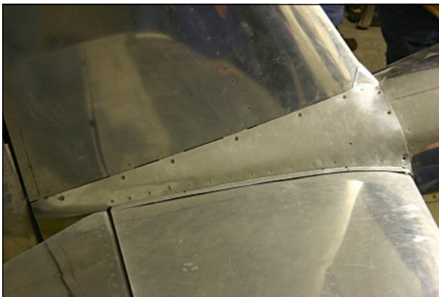
Greg fashioned Aluminum fairings for the horizontal-vertical stabilizer intersection.
