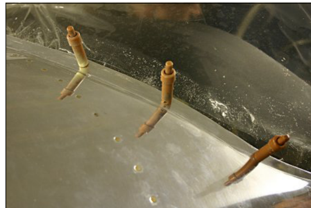
The boot-cowl to windshield intersection has a turned up flange to meet the Plexiglas.
