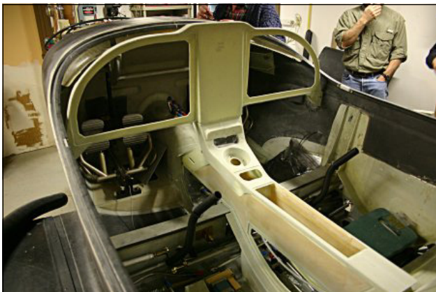
Dave demonstrated a reinforcement on the center console.
