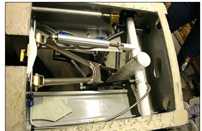
The landing gear weldments.
