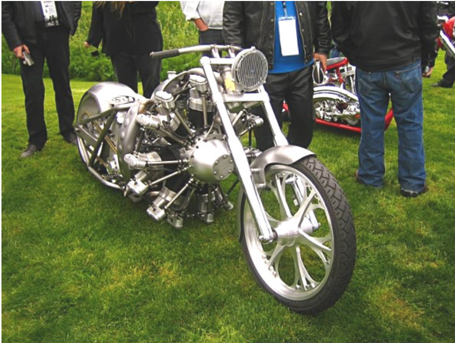
Yeah, it's a motorcycle—but it's an airplane engine. A Rotec R-2800.
