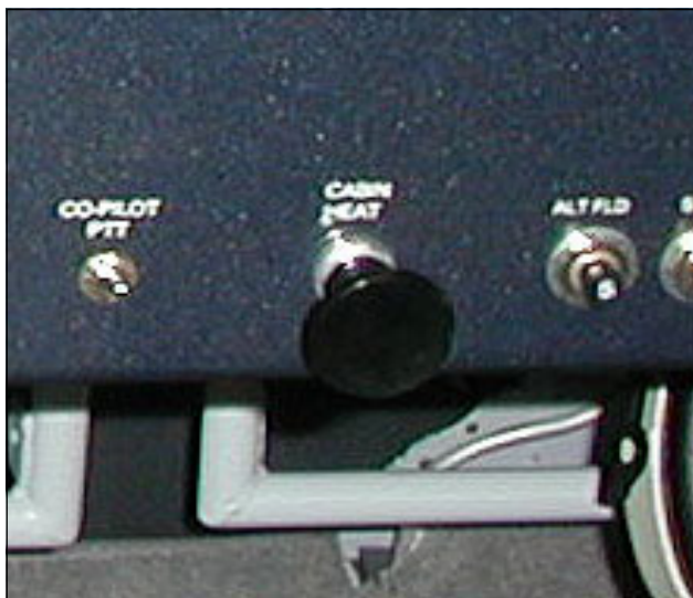
Left: The 'before' arrangement—the control is fixed to the main panel. Right: The 'after'—removing the two screws allows the cable assembly sub-panel to separate from the panel, allowing the panel to be removed without also pulling the cable.
