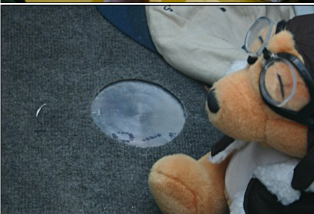
John Pallister's down-pointing camera port in his cargo area. He uses a D-SLR still camera, and a small video camera connected to a video monitor on his PDA at the pilot's position.
