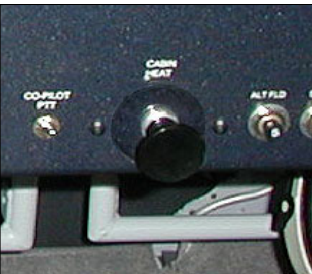
Left: The 'before' arrangement—the control is fixed to the main panel. Right: The 'after'—removing the two screws allows the cable assembly sub-panel to separate from the panel, allowing the panel to be removed without also pulling the cable.
