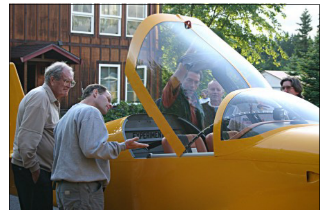
Dann's canopy slides back, disengages, then tips forward for loading bikes, etc, into the cargo space.
