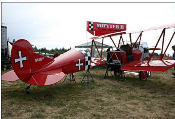
The Mifyter-II breaks in two behind the cockpit for transport.
