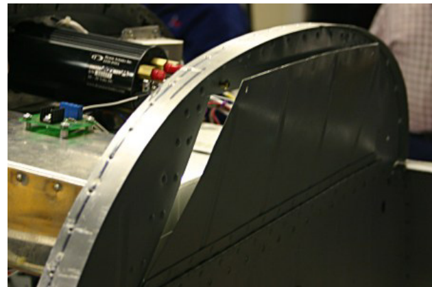
Ray included a hinged door allowing access to the forward side of his instruments.
