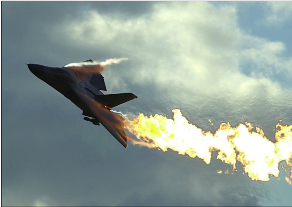
(Says Chris) I believe this is the old, hit the fuel dump and light the afterburner trick I have heard about being able to be done on the F-111. Photo from Christian Buhlmann via Dave Schwartz.
