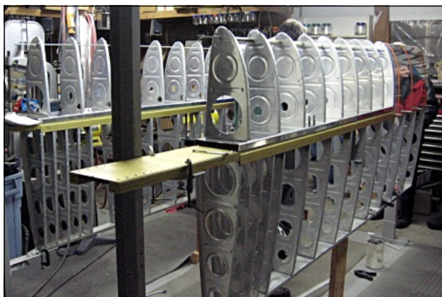
The wings — Doug's 37th set — are being built side by side.
