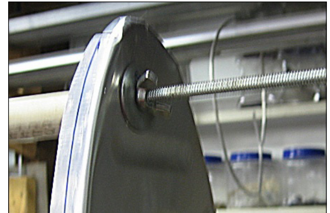
The nose ribs are spaced with sections of PVC pipe strung over a threaded rod.
