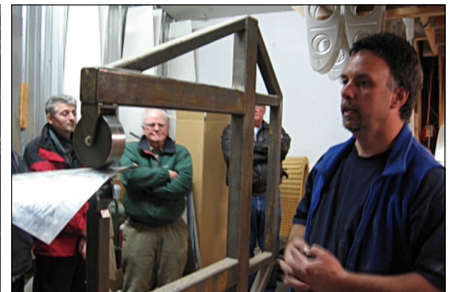
Doug demonstrates the stretching action of his English Wheel.
