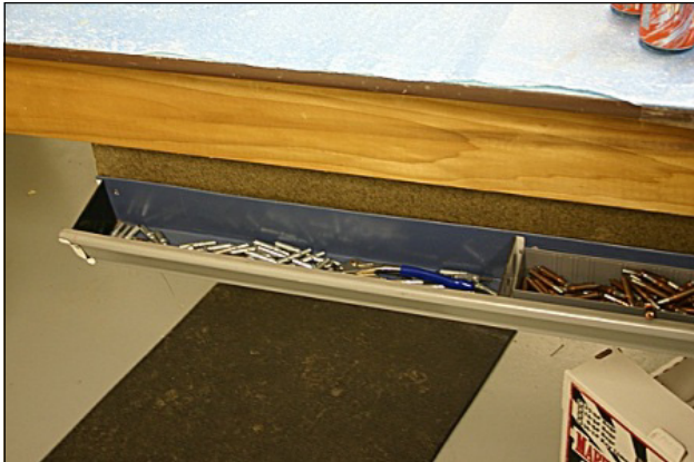
Rain gutter serves as a Cleco catch bin.
