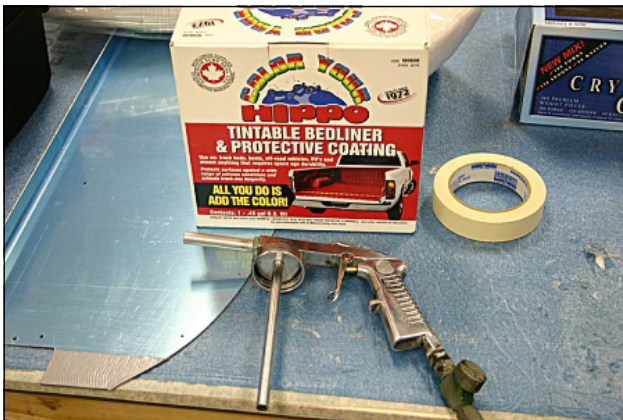
The brothers will use spray-on bed-liner for sound dampening.
