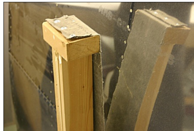
Web or carpet slings support the wings and fuse curves.
