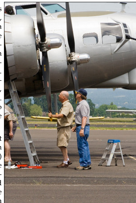
Checking the mag timing
