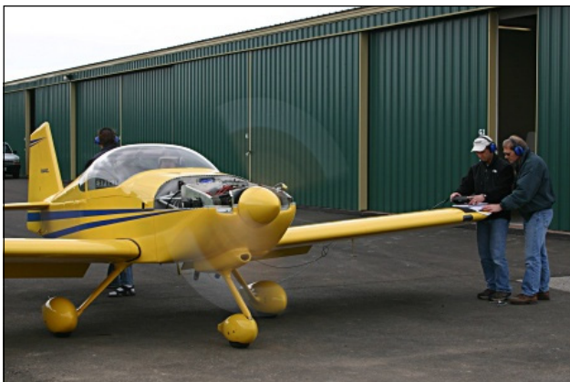
Randy Lervold and Len Kauffman, one of our two crack prop-balancing teams—members don't need to learn to use the equipment to have their props balanced, just make arrangements with Randy or Mike McGee for the alternate team.
