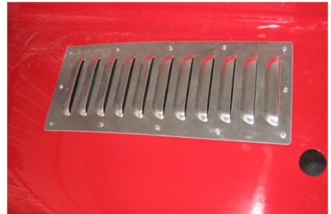
Rectangular holes are cut in the lower cowl below each cylinder bank. Then the louvers are attached with pulled rivets. The aluminum pieces conform well to the compound curve.
