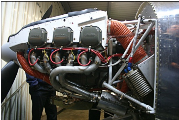
The flap actuating mechanism. Dan's all-glass panel. Left and right sides of the Aerosport IO-540 engine.
