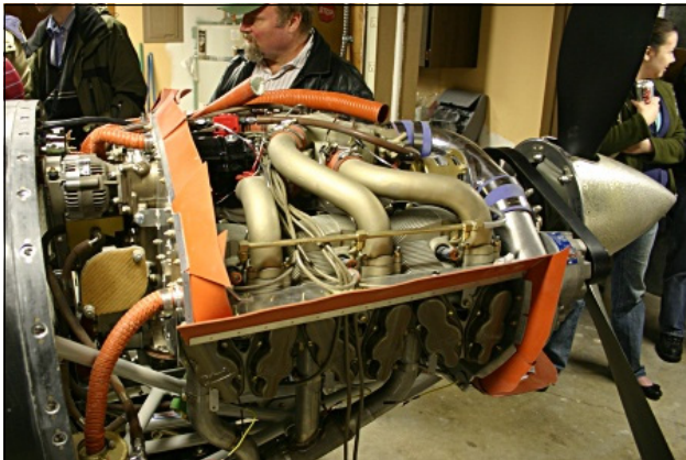
Dave's Lancair mounts a super-normalized Continental IO-550.
