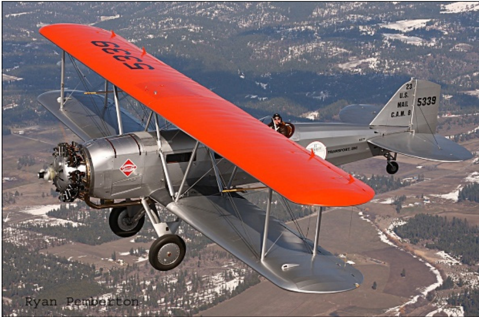
Ryan Pemberton The fabulous Boeing Model 40 of which we've been seeing occasional progress photos is flying now. A product of the Pemberton shop in Spokane, WA. Photo: Ryan Pemberton.
