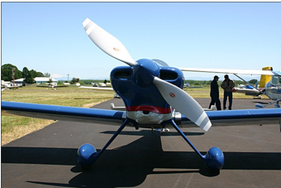
Rob Hickman's RV-4 is sporting a new experimental composite C/S Hartzell prop these days.
