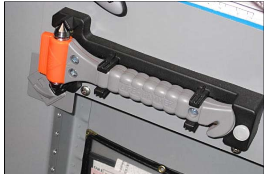
Life hammer — a blade for cutting harness webbing and hammer for breaking the canopy.
