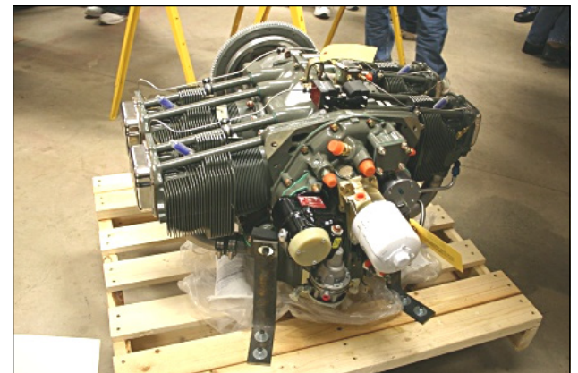
Top: The fiberglass canopy skirt was really tidy. Center: Classic Aero Designs interior. Note the molded side panels. Bottom: An Aerosport IO-320 will provide motivation.
