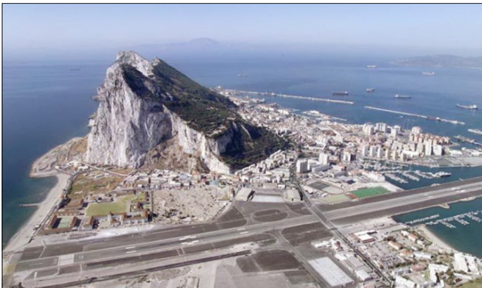
The runway at Gibraltar airport is crossed by ground vehicles traveling on Winston Churchill avenue. Traffic lights stop the ground traffic while aircraft arrive and depart. More photos on pg. 6.
