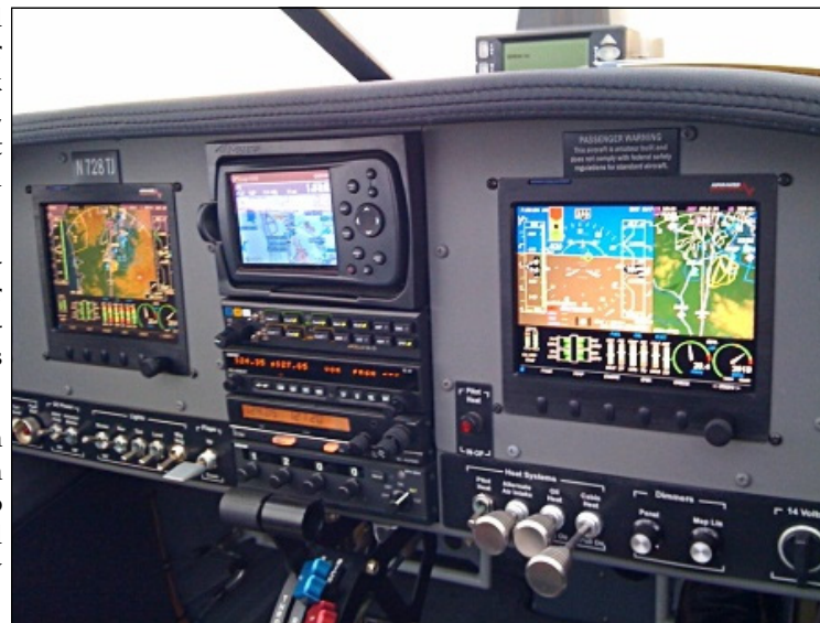
The panel of Joe and Tom's RV-7 features a pair of AFS 3400s.
