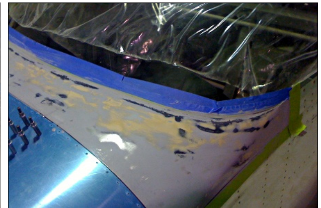
Leighton has been working with Roy Thoma, building up a really nice intersection in fiberglass and resin between Roy's RV project's cowl and canopy, shown here in four steps.
