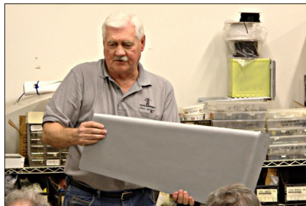
A vert-stab for a gyro-copter was crafted from a slab of urethane foam with the attach saddle formed over the member it will mount to, and a rudder pocket formed with a fir stick.
