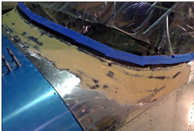
Leighton has been working with Roy Thoma, building up a really nice intersection in fiberglass and resin between Roy's RV project's cowl and canopy, shown here in four steps.
