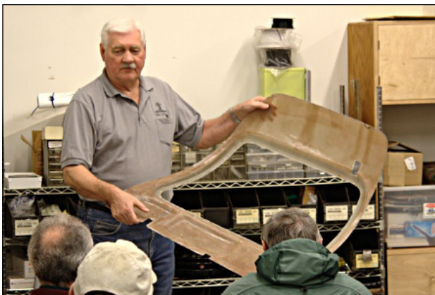
A panel was molded from an RV-10 door, with packing tape as the release, to be used by the upholsterer for cabin treatment.
