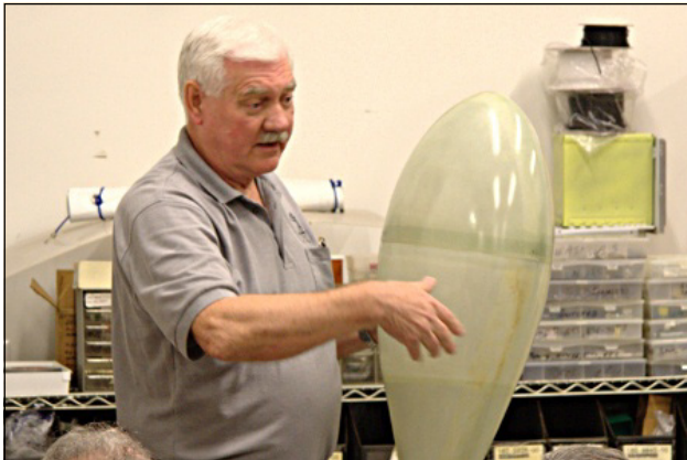
Leighton complemented the fiberglass work on stock RV wheel pants, but also had suggestions for how to dial in the joint between the front and rear halves.
