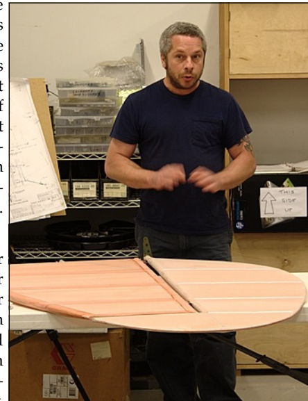
Trevor Lacy explains the covering sequence when using the Poly-Fiber process.
