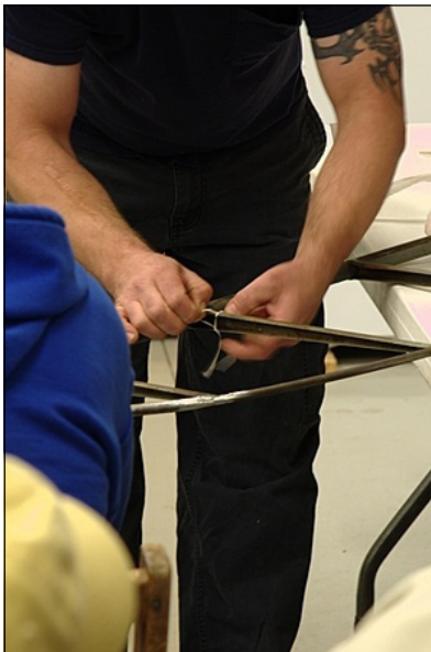
Trevor further explained the process with his demonstration aids including a quick rib-stitching demo.
