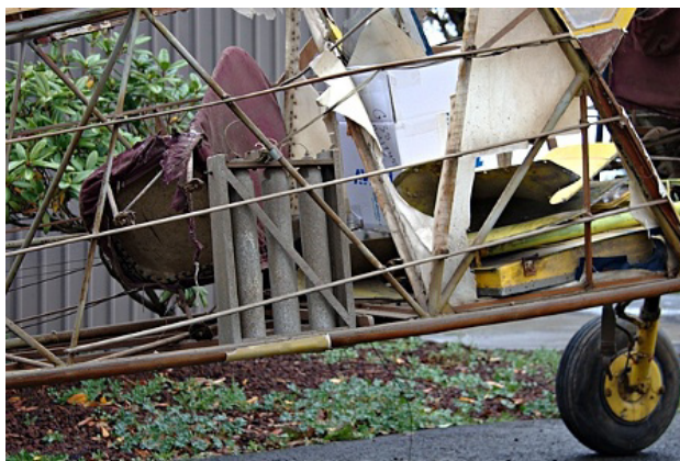
Two more shots of Bob Stark's C-38 project. This vertical tube structure behind the passenger compartment drew curiosity. It's a flare drop mechanism for lighting 'unlighted' fields.
