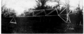
The simple yet sturdy fuselage structure of the Les-Wing Longship.
